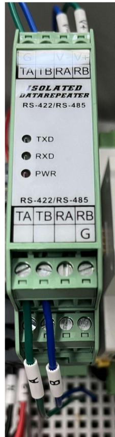
Wiring Connection-Lower Side
