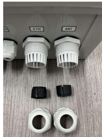
Waterproof plug with a cut
