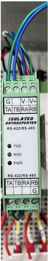
485 Repeater Whole View
