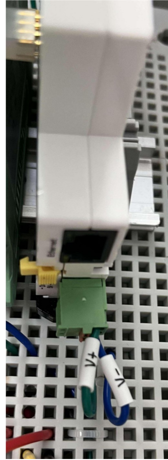
Power Supply Device DC Connection
